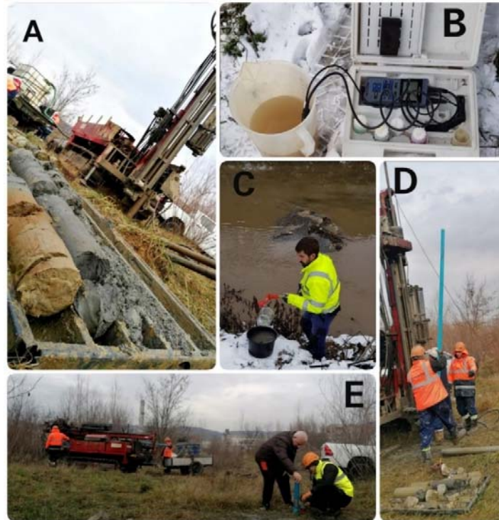
Figure 1: A. Making soil profiles using ROLATEC RL46L equipment. B. Determination of water pH on sampling site C. Collection of water samples from Someş riverbed, D. Installation of water sampling tubes at the level of soil profiles. E. Collection of water
