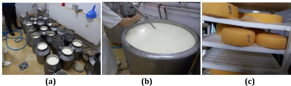
Fig. 1. Characteristic images for the main stages of the technological flow of processing the Dorna cheese: a-Qualitative and quantitative reception of milk, b-Preparation for coagulation, c-maturation chamber
