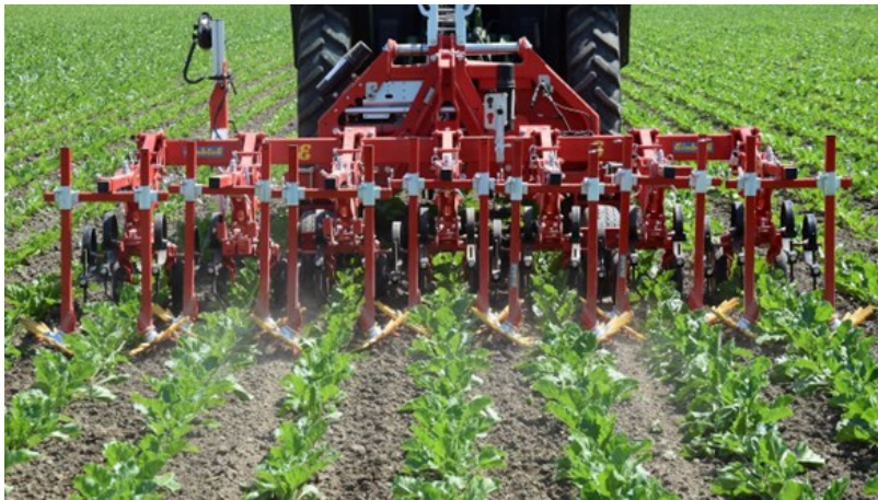
Fig.4. Precision hoeing with sensors and guidance intra-row and inter-row
